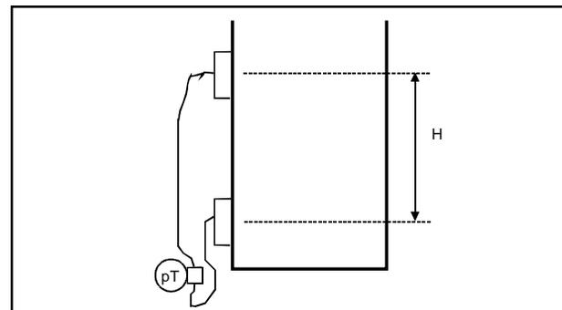
FIGURE 4 Density Measurement
