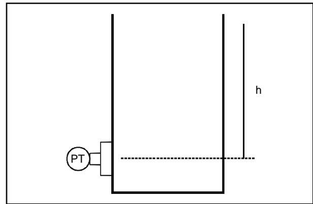
FIGURE 3 Hydrostatic Pressure
