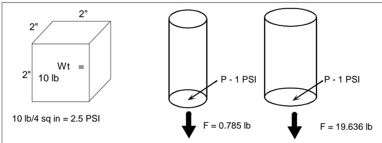
FIGURE 1 Pressure vs. Force Example
